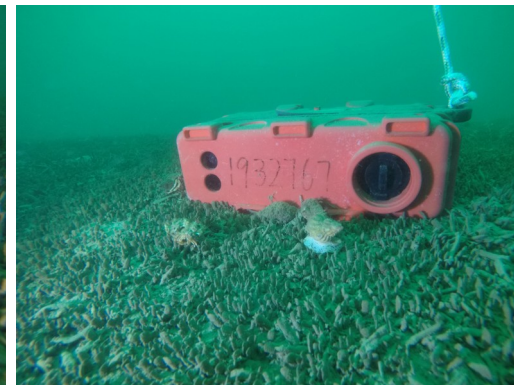
Seabed receivers : 4C GPR Nodes from Sercel
